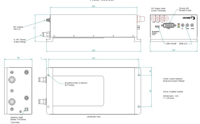
CTRL Control signals - : 26 way high density 'D' type
